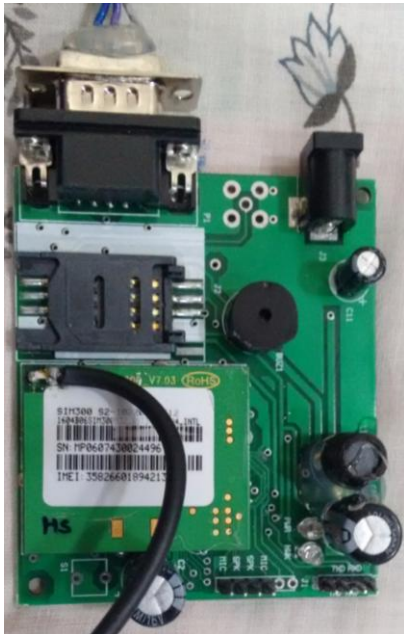
Figure 4: GSM Modem using SIM300 module
